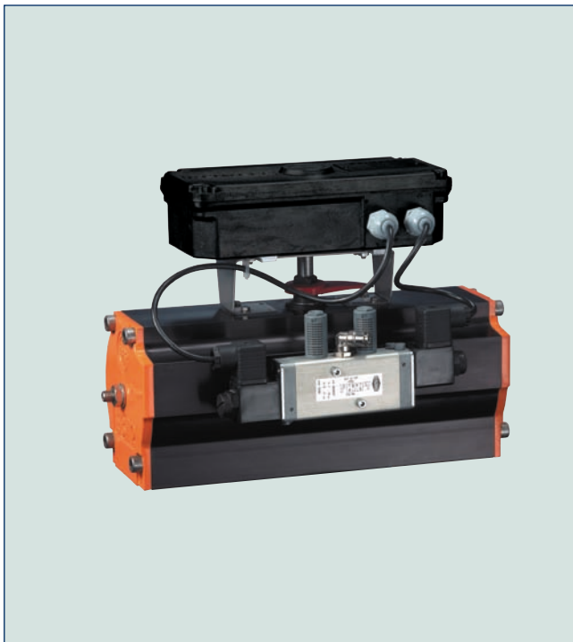
Pneumatic quarter turn actuator (double acting) with switch box NSK (Size II). Integrated proximity switches. Support acc. to VDI/VDE 3845. Compound coil pilot solenoid valve.
